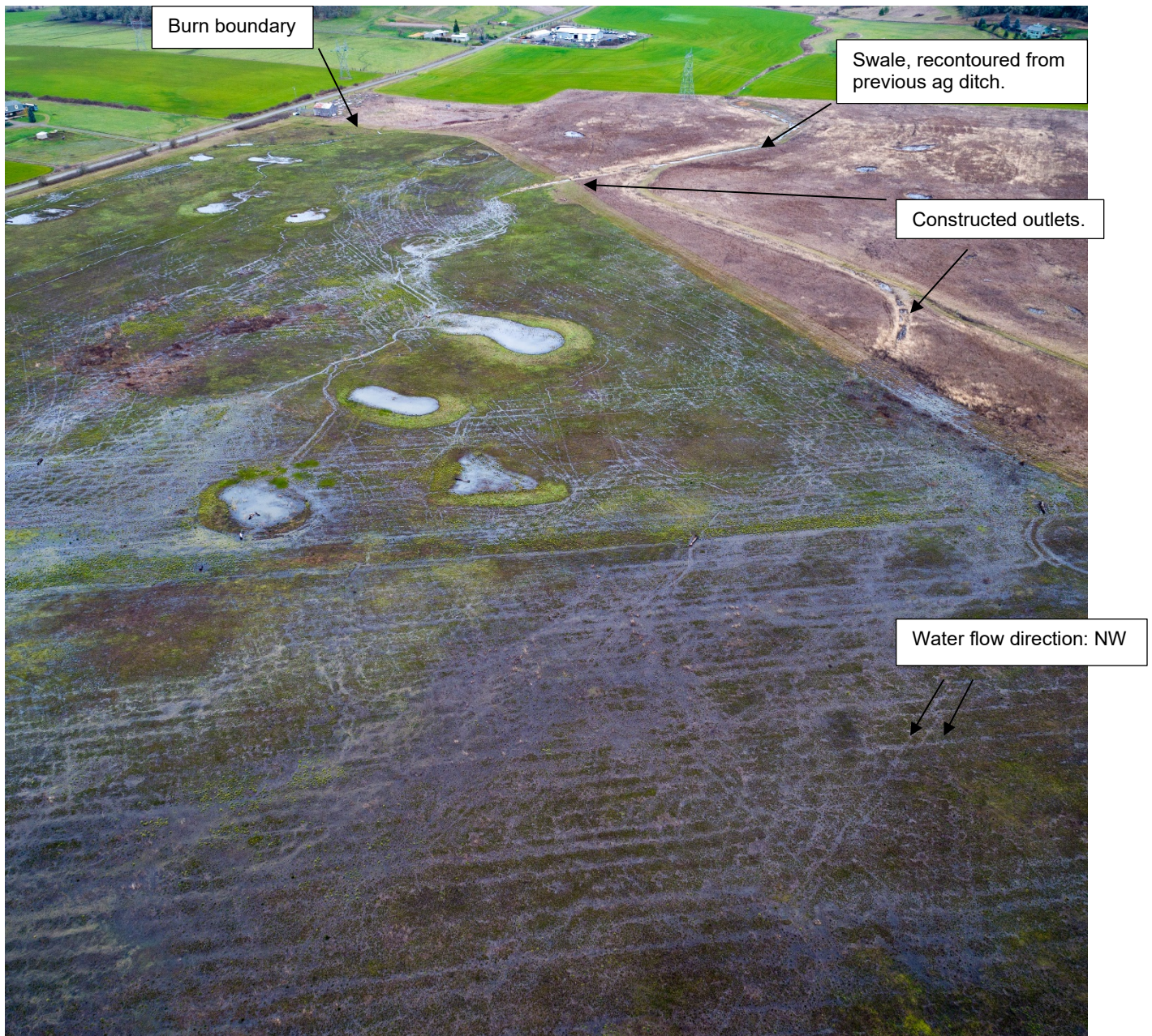
Fig. 3.5 Water is released from the former agricultural ditch, now recontoured into a broader, vegetated swale. Water released at outlets spreads across the well-vegetated, wet prairie of the East Phase. Water that does not infiltrate moves into pools in the East and West Phases and during storm events inundates the West Phase’s northwest corner. Surface water is visible in this January 2018 photo due to the prescribed ecological burn conducted in fall 2017. This photo shows successful achievement of PSH4.
