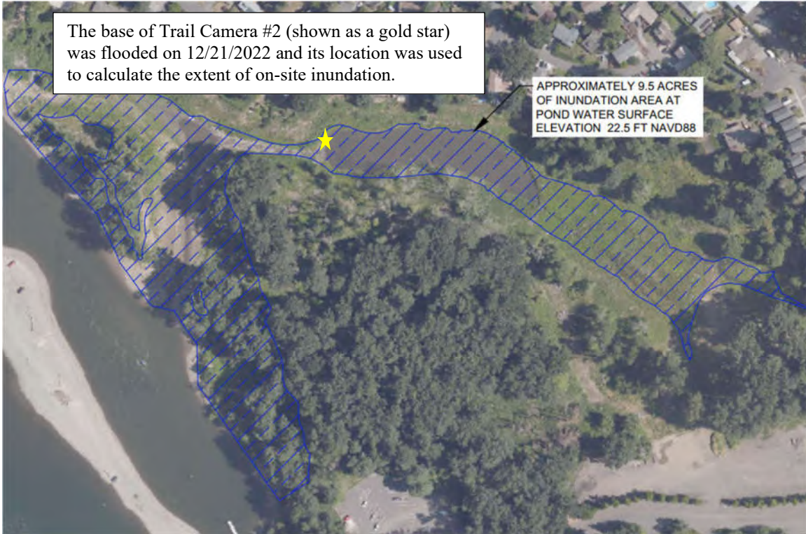
Figure 2-8: A high-water event observed on December 21, 2021 inundated approximately 9.5 acres of the site when the Oregon City gauge station was at 19.97 feet (NAVD88).
