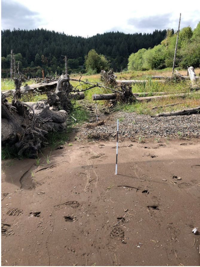
Photo 12 – Outlet, note approx. 6" sediment on 9/5/23
